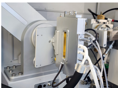
XRD原位冷热台适配赛默飞X-射线衍射仪
